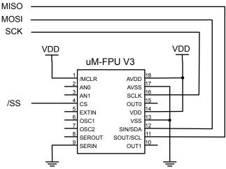
The clock signal is idle low and data is read on the rising edge of the clock (often referred to as SPI Mode 0).
