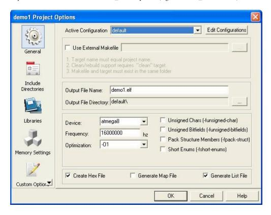
Note: Always confirm that the Device and Frequency are set correctly for the Atmel AVR microcontroller you are using.
