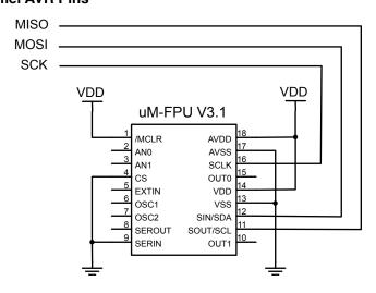
**SPI Pins for various Atmel AVR microcontrollers**
