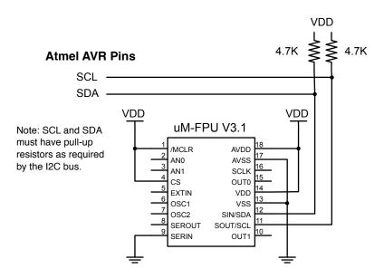
I<sup>2</sup>C Pins for various Atmel AVR microcontrollers
