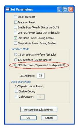
When this mode is selected, the SPI interface is automatically selected at Reset, and the CS pin is enabled as an active low chip select. The SOUT pin is high impedance when the uM-FPU V3.1 chip is not selected.
