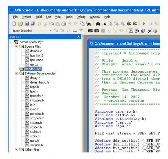
The following header files and include files are used by the FPU support software and must be in the search path:
